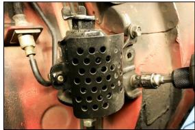
6. Using a 10mm socket wrench, remove the 2 bolts that secure the fuel filter mount to the chassis.
