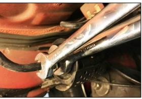
4. Using a 10mm socket wrench, remove the ground wire ring terminal bolt. NOTE: This could be found on any one of the 3 bolts shown.
