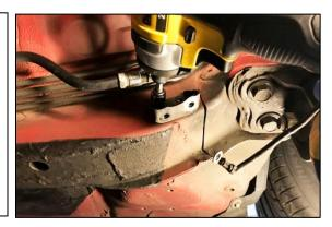
7. From the engine bay, remove the fuel rail feed line banjo bolt.
