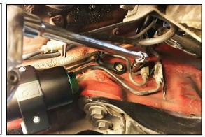
11. Relocate and secure the electrical ground wire ring terminal to the mounting boss, as shown.
