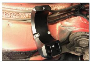
9. Temporarily install the Radium fuel filter (not included) and upper clamp to the lower mount using the 2 socket head screws and a 4mm Allen wrench. Do not torque these bolts yet.
