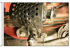
5. Using a 10mm socket wrench, remove the 2 bolts that secure the fuel filter to the fuel filter mount.
