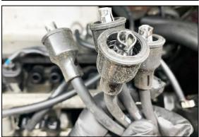
8. Gently pry the cable(s) from the fuel rail stays. NOTE: The first 4G63 engine variations will have 2 cables.
