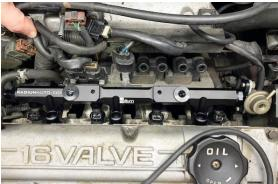
17. Place the 3 phenolic washers onto the 3 provided M8x1.25mm bolts.
