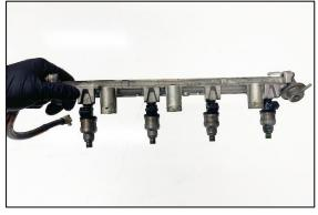
10. Be sure to find the lower injector O-rings as the will sometimes get stuck in the cylinder head. Inspect the condition of both the upper and lower injector O-rings and replace if necessary.
