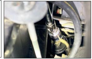
6. Using pliers, remove the return hose from the fuel pressure regulator. Catch any fuel that may spill from this connection and properly dispose.
