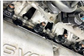
12. When installing the 3 mounting feet to the fuel rail, apply a high strength thread locker to the six M5x0.8mm bolt threads. Secure using a 4mm Allen wrench.
