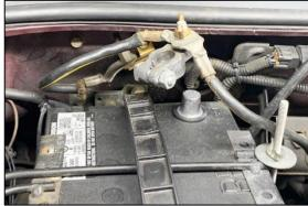
5. Find the fuel filter mounted on the firewall.
