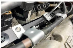
25. After everything is reinstalled in a reverse order, cycle the key a few times (without starting engine). This allows the fuel pump to prime the system.
