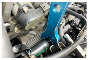
24. Position the cable bracket stays 180 degree from how they were oriented with the OEM fuel rail. The single cable bracket variation is shown. The early dual cable bracket variation will slightly differ.
