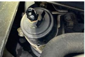
15. Install fittings to the 4 ports. Lubricate all O-rings prior to securing.
