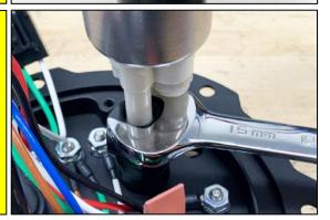
15. Reinstall the fuel pump bracket. Allow the "fuel sensor" connectors to exit the pump bracket in the direction depicted (top of picture). This will setup for easier connections in a later step.
