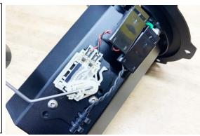
24. Using a 2.5mm Allen wrench, remove the pressure sensor hold-down bracket.
