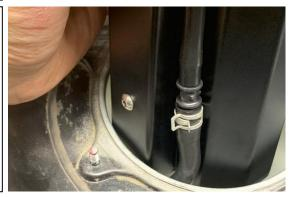
27. When dropping the fuel hanger down into the tank, be sure components such as the fuel level float, crossover hose (shown), sensor connectors, etc. do not get hung up.
