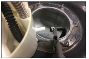
5. To remove the fuel level and fuel temperature sensors from the OEM fuel pump housing, first depress the thumb tab and unplug the larger 4-wire connector from underneath the top plate. Next, pry and pop the fuel temperature sensor probe out of the locking tabs.
