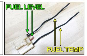
21. Strip all 4 wires from the fuel level sender and fuel temperature sensor. Next, crimp the 4 included terminals to each wire using a tool such as Molex 63811-1000 hand crimper. Slide the terminals into the plastic plugs until a "click" is felt. Polarity is not critical.
