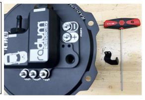
25. Inspect the condition of the OEM gasket and replace if necessary (Mitsubishi MN139931).
