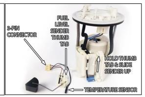
6. To install fuel pumps, the fuel hanger must be partially disassembled.
