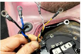
32. After installing the ring terminals to the appropriate studs, tighten the insulating acorn nuts.
