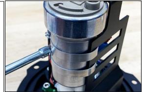
17. If using 2 pumps, install the provided connector harness ring terminals to the "PUMP2" wiring studs underneath the top plate. Tighten the lock nuts with a 3/8" wrench.
