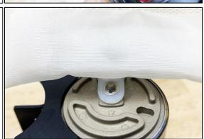
19. When dropping the assembled unit back into the collector box, the filter sock(s) might need to be folded for best clearance. Reinstall the collector box mounting screws.
