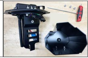
7. To remove the fuel pump bracket, unscrew the 3 socket head screws using a 4mm Allen wrench. NOTE: the fuel pump bracket may be a different color depending on the kit purchased.
