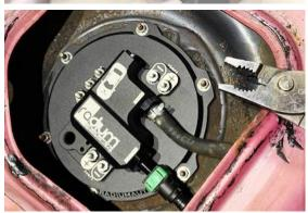
29. Send the OEM harnesses and pressure sensor from the interior back through the sheet metal hole and on top of the fuel tank. Reseat the rubber grommet.
