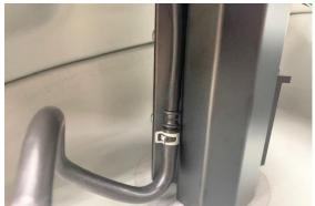
28. Reinstall the OEM M5 flange nuts using an 8mm wrench. Tighten to factory specs in steps using an alternating crisscross pattern.
