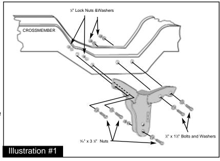
7. Now install a  $\frac{1}{2}$  x  $1\frac{1}{2}$ " supplied bolt, labeled as "**B**", through new bracket and crossmember. Pivot the bracket down so that tab is flush against crossmember lip. Torque these bolts to specifications. Drill  $\frac{1}{2}$ " hole, for bolt labeled as "**C**", and install supplied  $\frac{1}{2}$ " bolt through tab on new
