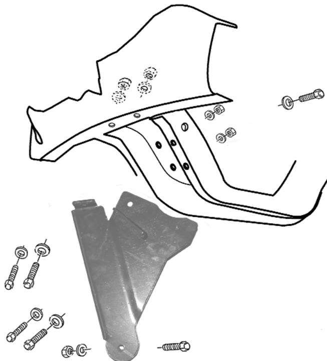
9. To install new right axle beam bracket, start bolts (1/2 x 2") through bracket, cross member and then backing plate, so that the washers and nuts will be on the cross member side next to front bumper. Swing up axle beam and install new 9/16 x 3 1/2" bolt. Tighten all bolts.
