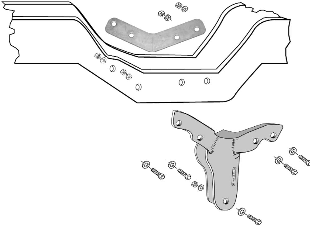
10. Install new radius arm brackets, and bolt original brackets to the new ones (7/16 x 1 1/2"). The bolt holes on the frame and radius arm cross member will need to be drilled out to 1/2". Double the amount of washers are included so that a washer is used under each bolt head and another one against the nut. Tighten all bolts.
