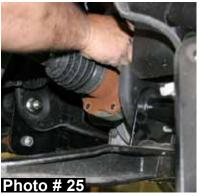
30. Attach the OEM outer tie rod ends to the new Skyjacker steering knuckles using the OEM hardware. Mark a line along the brake caliper mounting surface of the new steering knuckles & trim the OEM brake dust sheilds for proper brake caliper fitment using a cut off wheeel or similar tool. (See Photo # 28 & # 29) Reinstall the OEM brake rotors & OEM brake calipers using the OEM hardware.
