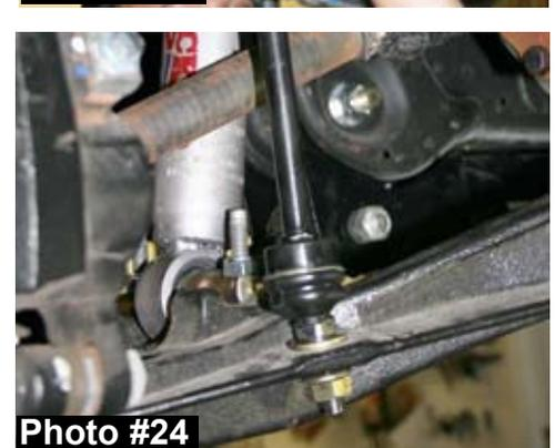
26. Install the new Skyjacker anti torque link by installing the bushing in the eye of the assembly. Attach the eye at the new Skyjacker crossmember using the 1/2" hardware supplied. Adjust out & attach the rod end to the lower ear on the differential using the inserts & 9/16" hardware supplied. Once installed, tighten the jam nut. (See Photo # 25)
