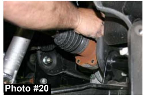
21. Attach the ABS line to the steering knuckle using the 5mm x 12mm bolts supplied.
