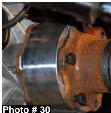
Driver side shown with 3.35" cv-shaft spacer.
