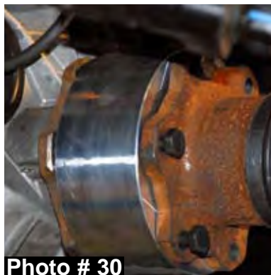
Driver side shown with 3.35" cv-shaft spacer.
