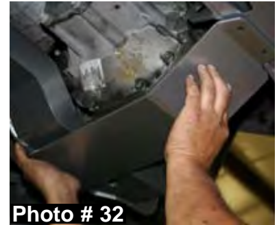
Passenger side shown with one 15/16" C.V. spacer.
