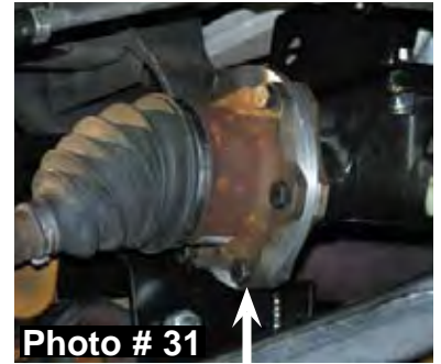
Passenger side shown with one 15/16" C.V. spacer.
