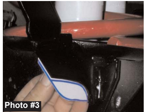
Photo #3 The above picture shows the removed portion of the lower track bar mount.
