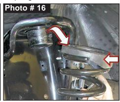
NOTE: Installing Coil Seat Metal Spacers: Proceed to Step 15.
