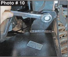
11. Remove OEM bump stop using adjustable channel lock pliers or a flat screwdriver.
