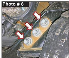
10. Install Skyjacker # TB1120-B Track Bar Bracket to the OEM crossmember. Insert supplied 9/16" x 3" Fine Thread Bolt with 9/16" SAE Washer from front-to-rear through bracket \crossmember mount. Place # D260PSS-S Anti-Crush Spacer (0.938" Long) inside bracket. Insert bolt through bracket \crossmember mount.
