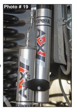
21. Connect Skyjacker front shock at upper shock tower mount using a 18mm socket\wrench.
