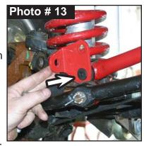
23. From # HB-TBA60 Hardware Bag, install Skyjacker Track Bar rod end by following the hardware pictured. (See Photos # 14 & # 15) Being sure to keep the rod end square (parallel) with the frame mount.
