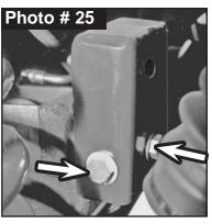
10. Install Skyjacker rear coil spring. Be sure coil spring is seated properly at lower axle mount by rotating the coil until the pigtail hits the spring stop. **Note:** Be sure OEM upper coil spring isolator is properly aligned with coil & upper coil spring mount.
