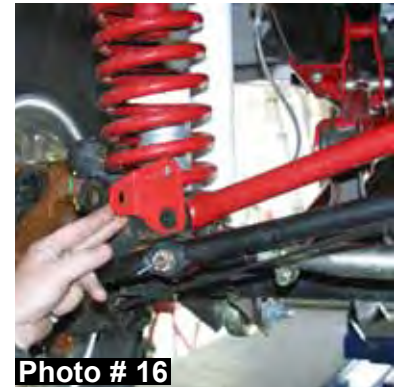
5/16" x 3/4" thread cutter flange bolt.
