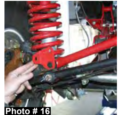
5/16" x 3/4" thread cutter flange bolt.
