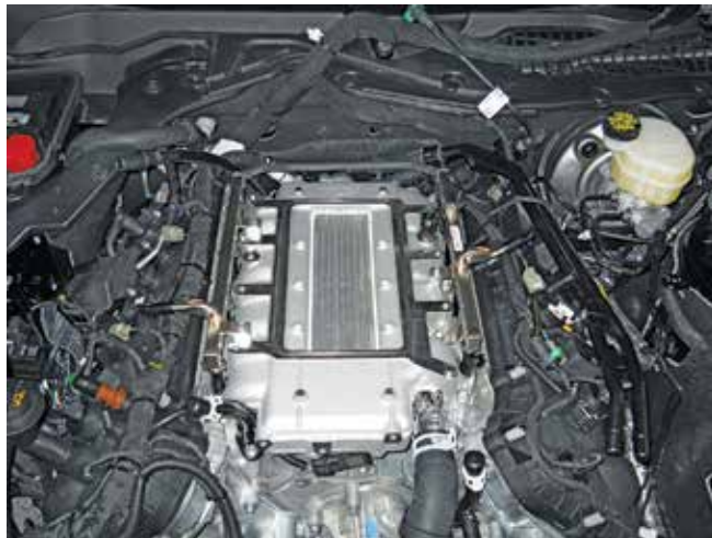
14. Connect the eight (8) fuel injector electrical connectors.
