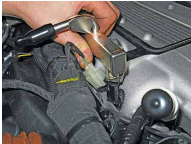
15. Plug in the connector to the fuel pressure sensor on the fuel rail.
