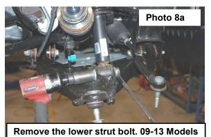
14. Lower the jack to let the lower control arm and knuckle swing down so the strut can be removed.
