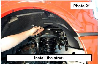
studs back into the barpin on the lower mount of the strut. It may be necessary to hit the top of the strut with a hammer to seat the splines before tightening the factory nuts with a 18mm. See Photo 22.
