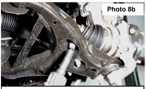
Remove the lower strut bolts. 14-20 Models
