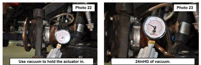
37. With vacuum still applied to actuator. Measure the depth of the CV shaft threads protruding through the hub
