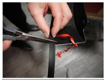
**STEP 4:** Trim any unnecessary extrusion and discard.
