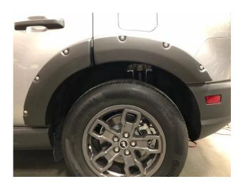
**STEP 12:** Repeat installation method for other side. Double check the front Fender Flares to make sure all clips are securely fastened. Your installation is now complete. Do not use abrasive cleaners.
