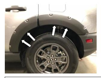
**STEP 10:** As performed prior in Step 6, Pull red tape liner back 1-1/2 on both fender flares. Place the Fender Flares onto the vehicle and fit into the correct position following the contours of the vehicle body. Use 4 of the retaining clips provided and secure the Fender Flare to the body starting at the positions pointed out above. Be sure the clips "snap" securely into the slotted hole of the Fender Flare.
