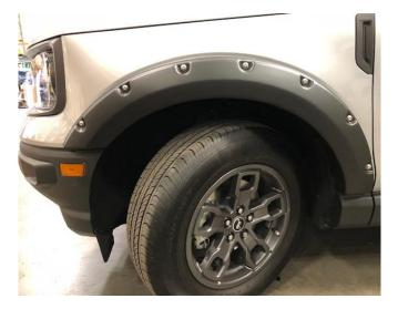
**STEP 8:** Repeat installation method for other side. Double check the front Fender Flares to make sure all clips are securely fastened. Your installation is now complete. Do not use abrasive cleaners.
