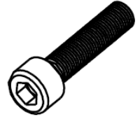
M6 x25 Socket Cap Screw x8
