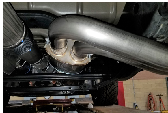
Detail 10a: Tailpipes installed to muffler.
