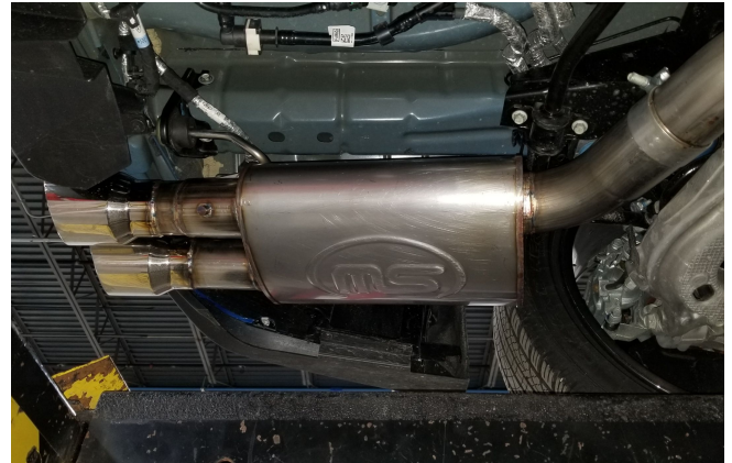
Detail 12a: Left muffler assembly installed
