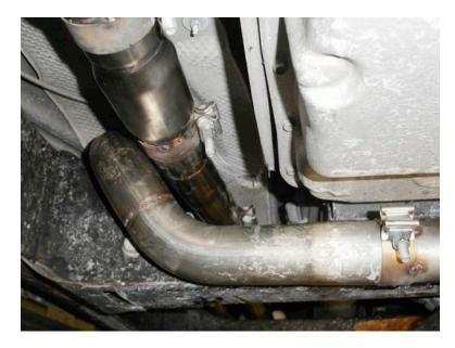
17. Place 2-1/2" clamps on the X-pipe or Y-pipe as provided in your kit and slide onto the leadpipes. The X-pipe or Y-pipe will not sit exactly level for a proper installation. The picture below shows the X-pipe properly positioned from the rear of the truck. The Y-pipe connects to the lead pipes exactly as the X-pipe.
