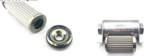
3 – The cap with the spring is the INFLOW! The magnet should be readily visible on the filter element and the smaller diameter of the spring presses into the dish of the filter.
