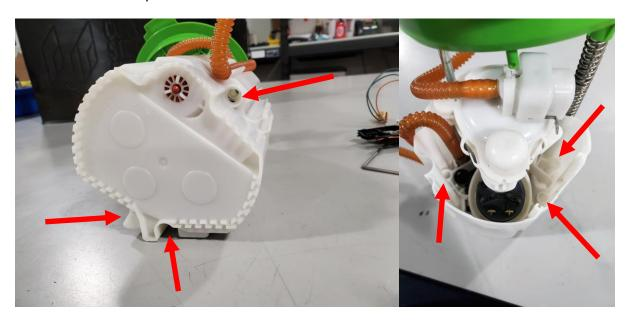
4 – Remove the top hat support posts from the bucket and remove the center section from the bucket. Due to manufacturing tolerances there may be some remaining plastic remnants holding the module together, rocking the center section and flexing the bucket gently from side to side should loosen any remaining plastic weldments. Once separated remove any plastic debris from inside the bucket, and cleanup the 3 areas you drill through to remove any jagged plastic bits.
