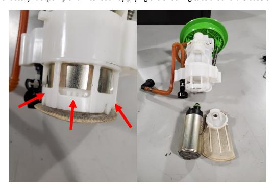
6 – Remove the spacing cage the OEM pump slid into. There are 4 locking tabs around the diameter of the module. The cage will not be reused if damage is done during removal.
