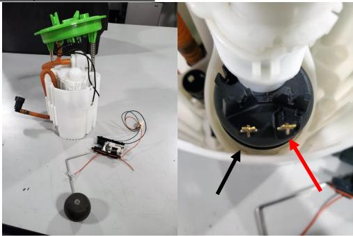
2 – Unhook the venturi hose connection from the side of the bucket, and compress and remove the e-clip that holds the top hat to the bucket.
