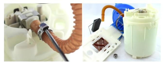
4 – Removed the bucket cap by lifting the four tabs around the top (circled in green), the pump will come out with the cap with a gentle pull
