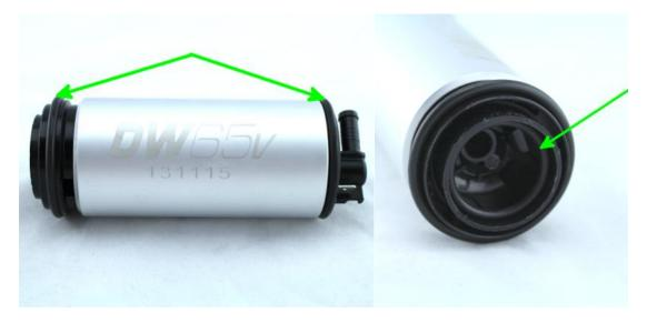
5a – The proper location for the larger lower O-ring is below the lip and leaves the rectangular port on the cap exposed (circled in green)
