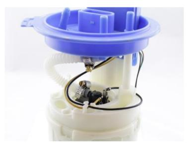
9 – AWD models will connect the factory venturi/siphon tube to the small outlet barb on the top of the fuel pump.
