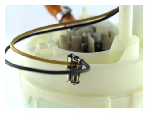
2 – Remove the screws that attach the top of the assembly to the bucket, these can be either a 7mm hex or T20 Torx
