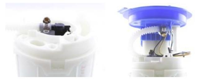
8 – Reinstall the top and connect the wires to the pump
