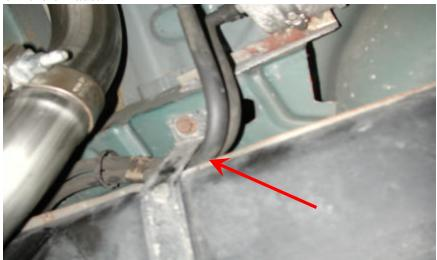
14. Please view photo below of suggested clearance of passenger side tailpipe to the passenger side of the gas tank.
