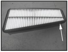
Step 7 Remove the factory seal from the perimeter of the filter.
