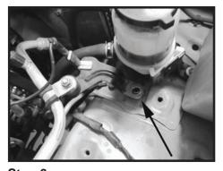
Reposition the A/C line bracket to line up with the hole on the power steering reservoir. Do not fasten it right now this will be done in a later step. You may need to loosen the nut on the rubber isolation mount allowing you to turn the bracket. If so make sure you tighten the nut back up after positioning.
