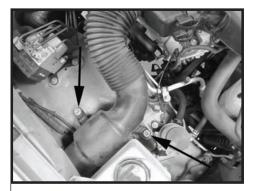
Step2 Remove the two screws securing the resonator.
