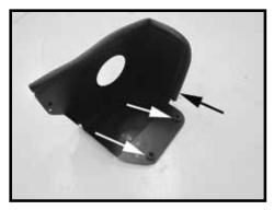
Step 11 Install the rubber bulb seal, this may require trimming to the correct length. Install the grommet removed from Step 8.
