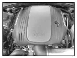
Step 16 Install top engine cover. Position the breather hose so it does not rub on cover.
