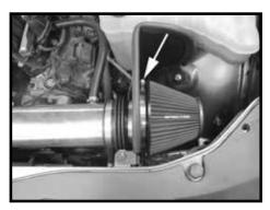
Step 15 Install the filter on the velocity stack adapter and fasten it securely. If required rotate the velocity adapter so the filter will fit without any fitment issues.
