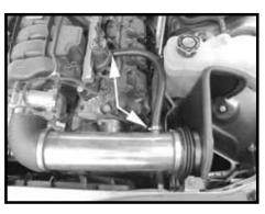
Step 14 Install the breather hose on the hose fitting on the engine and intake tube. Fasten it in place with the provided hose clamps.
