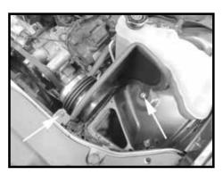
Step 10 Install the heat shield into the vehicle. Reuse the factory bolt from Step 5 and use the supplied hardware for the rubber insert.
