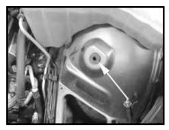
Step 9 Install the rubber insert in the hole located on the inner fender.
