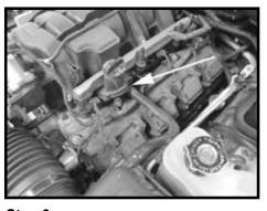
Step 3 Remove the breather hose from the intake manifold.
