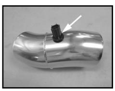
Step 6 Install the supplied grommet into the intake tube, and then install the IAT sensor into the grommet.
