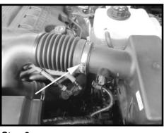
Step 2 Disconnect the electrical connector on the Intake Air Temperature (IAT) sensor.
