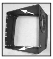
Step 8 Then install the 2 small pieces of 1/16" gap seal on the bottom of the heatshield as shown.
