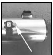
Step 12 Insert and fasten the pressure sensor onto the Spectre Performance intake tube with the provided hardware.
