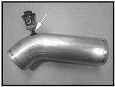
Step 13 Install the provided grommet into the Spectre intake tube then, install the filter minder into the grommet.
