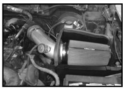
Step 20 Make sure that all clamps and hardware are fully tightened. Reconnect the battery cable and start the engine and let it warm up. Shut it off and inspect the installation once more for any loose clamps, wires, or hardware. Test drive & enjoy! Your installation is now complete. Periodically check all clamps and brackets.
