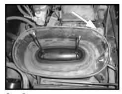
Step 5 Loosen the nut that secures the lower air cleaner assembly as shown.
