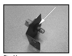
Step 14 Install the provided grommet into the air temperature bracket and then install the air temperature sensor into the grommet.
