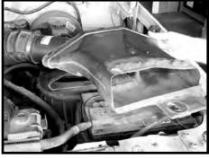
Step 2 Loosen and remove the bolt on the radiator core support, then remove the air inlet duct as shown.
