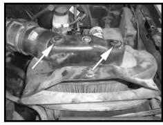
Step 3 Loosen the screws that secure the air cleaner top as shown.
