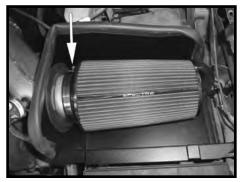
Step 18 Install the Spectre air filter and secure with provided hose clamp.
