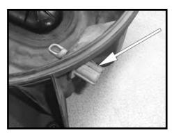
Step 7 Remove the air temperature sensor by turning it a 1/4 turn, then pull the sensor out of the lower air cleaner assembly as shown.
