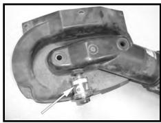
Step 12 Remove the filter minder from the stock air box.
