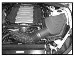
Step 5 Lift the entire air box assembly out of the engine compartment.
