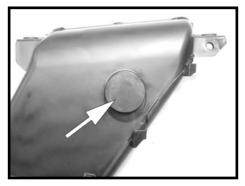
Step 7 Install the provided plug into the hole from the resonator into the fresh air duct.
