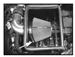
Step 14 Install the air filter onto the velocity stack and secure with the provided hose clamp.
