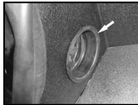
Step 15 Push fresh air duct through bottom hole in heatshield.
