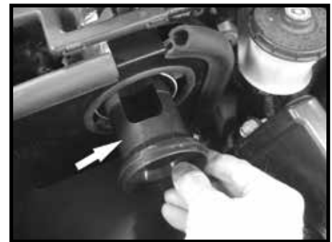
Step 16 Install MAF calibration sleeve into intake tube. Note; This calibration sleeve must be used or vehicle will not perform correctly.
