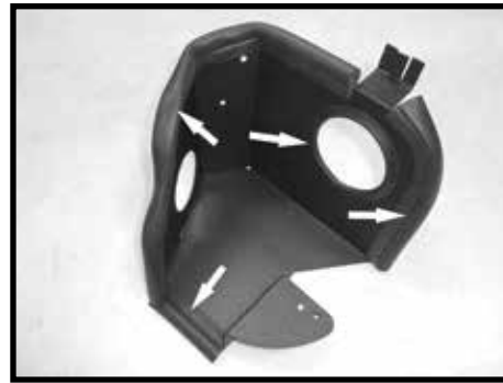
Step 12 Install edge trim onto heatshield as shown. Some trimming may be necessary.
