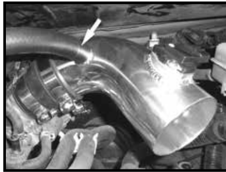
Step 11 Install intake tube into reducer couple and slightly tighten at this time. Push one end of new PCV hose onto intake tube.
