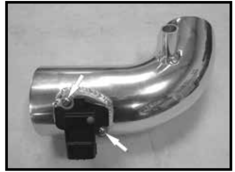
Step 10 Install MAF sensor into the Spectre air intake tube with provided hardware.
