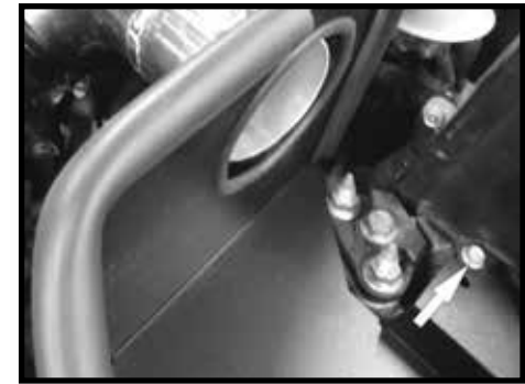
Step 13 Slide heatshield into position and install inside bolt.
