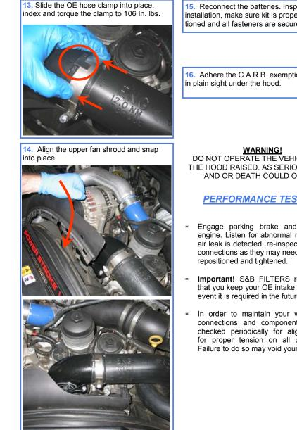
Reconnect the batteries. Inspect your installation, make sure kit is properly positioned and all fasteners are secure
