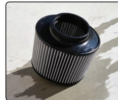
**Gently shake Filter to Remove Excess Water**
