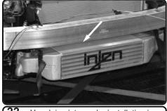
**22.** Your Injen intercooler installation is now complete. Make your final adjustment and make sure all your nuts, bolts and clamps are secure. Reinstall the rest of the bumper components in reverse order.
