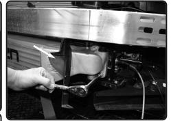
**21.** Tighten the Passenger and driver side intercooler using 12mm socket or wrench.
