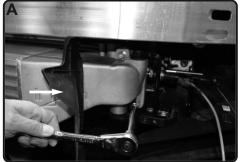
**20.** Re-install the OEM screws and secure the injen intercooler.
