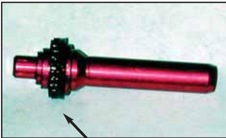
Remove seal from piston.
