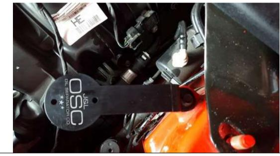
Use the supplied screws to mount the J&L Separator assembly to the J&L bracket routing the "O" hose ("O" Side of can) down toward the engine mount to connect to the PCV, and the T hose ("C" Side of can) under the intake for the fitting behind the throttle body.
