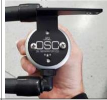
Locate the stud on the driver side firewall where this will mount. Pry off OEM hose holding clip, use the supplied 10mm nut and secure the oil separator assembly to the stud and FLIP and reinstall the holding clip. Route Oil Separator hoses UNDER OEM lines and across the
