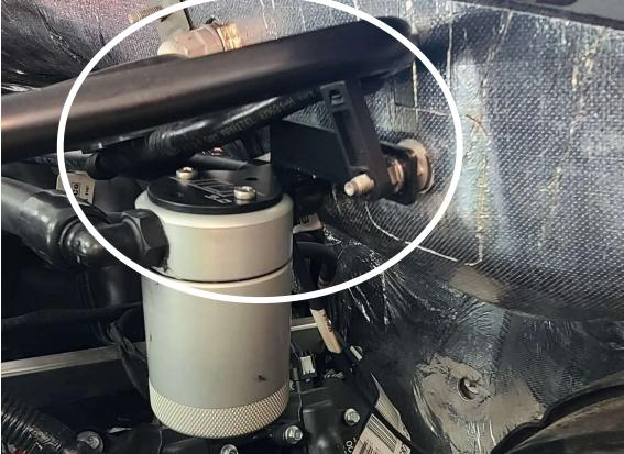
Install REAR/LONGER hose to the PCV connection on valve cover Install FRONT/SHORTER hose to fitting behind throttle body
