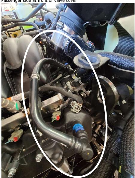
Pull wire clip on intake UP and pull intake tube out of the way
