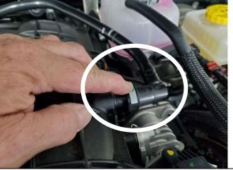
Use the supplied 10mm bolt to mount the J&L bracket to the threaded hole in the driver side of the Jeep shown here:
