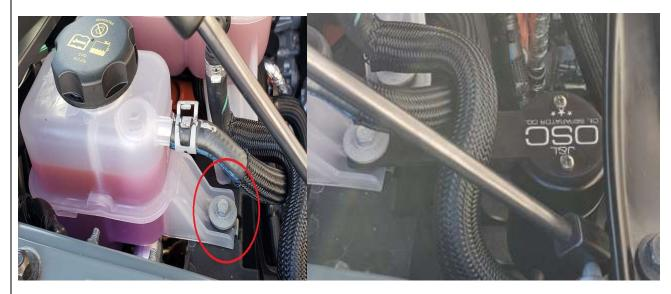
Page 1 of 2 1-27-23 The shorter hose will connect to the PCV valve on the valve cover.
