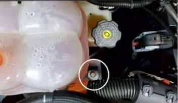
With this bolt removed, you can pivot the tank off the front stud on the fire wall. You will install the J&L assembly onto this stud with the supplied nut. Tighten nut down and reinstall coolant tank and bolt.
