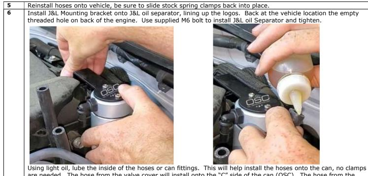
are needed. The hose from the valve cover will install onto the "C" side of the can (OSC). The hose from the intake manifold will install onto the "O" side of the can.
