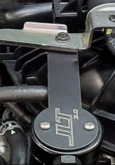
Take the shorter of the two J&L hoses. This line will run to PCV Valves on the valve covers from the "O" (OSC) side of the J&L oil separator. Start from back of engine and route long line under coolant line and breather line. Use light oil inside hose end and lightly oil connection on oil separator and PCV Valves. This will help to slide hose all the way on to their connection points. Once hose is attached slide clamp up on the PCV fittings with pliers.
