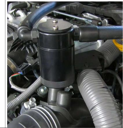
8 Reinstall engine cover, slide cover into place under J&L hose. The cover attaches to the horizontal bar and into two separate grommets. Be sure cover clears oil separator bracket, you will need to now tighten the bracket bolt. The cover will need to be shifted back out of the way to tighten this bolt.
