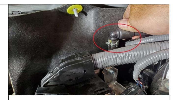
The hose with the short rubber section will connect to the intake manifold fitting, be sure to preinstall the hose clamp and ensure the screw of the clamp is on the upward side of the hose to allow for easier tightening of this clamp. Tighten clamp and pull-on hose to ensure it's tight enough to not pull off, the intake manifold is pressurized by the turbo's so this needs to be tight enough to withstand the pressure!
