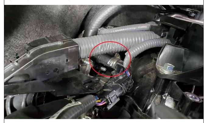
Reattached wiring harness to support.
