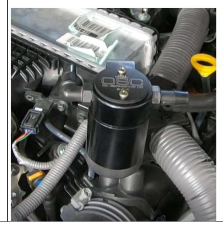
Connect hoses to oil separator, use light grease or oil inside of the end of the hoses (a Q-Tip is useful here). Be sure to slide the dress up ends onto the hose ends before installing hoses onto the oil separator. The hoses should bottom out to the base of the fittings!
