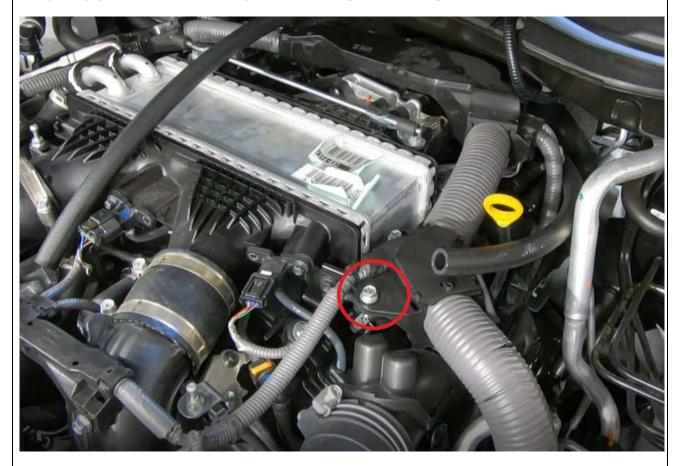
Mount J&L Oil Separator to mounting bracket with supplied screws.
