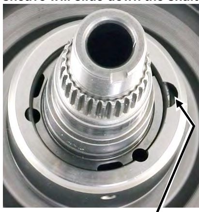
Line up Hump on snap-ring to half-moon groove in sheave.
