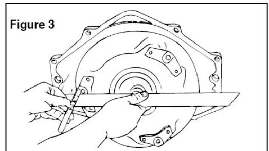
Measure the depth of mounting pad face (A) from the mounting flange face. Notice that the right hand that is holding the straight edge is also pushing the converter in toward the transmission.
