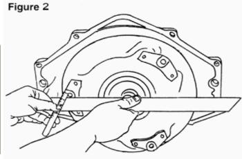
Measure the depth of mounting pad face (A) from the mounting flange face. Notice that the right hand that is holding the straight edge is also pushing the converter in toward the transmission.
